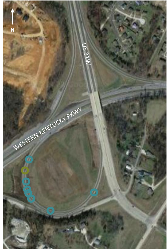
WKP Exit 136 (US 31W): Add high friction surface treatment on US 31W southbound to WKP eastbound ramp (right).
